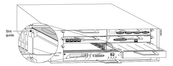
Note: This adapter alignment applies to any port or service adapter.
